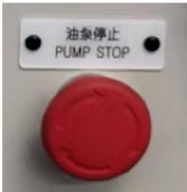
Emergency button can stop the pump at once when happen any accident.
