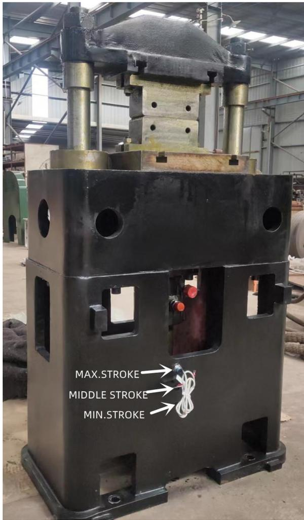
The press allow to adjust the stroke according to working requirement.
