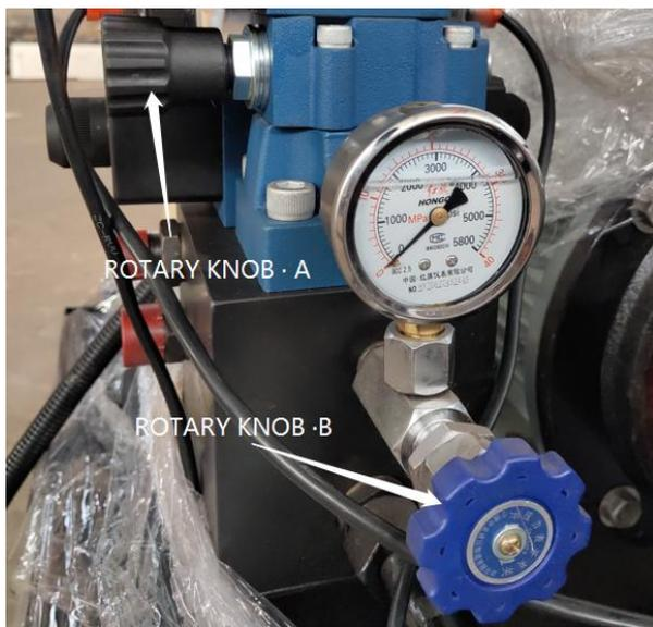
Oil pressure gauge to show system pressure should be 25MPa.
